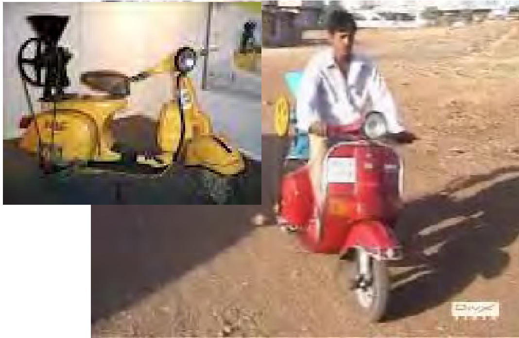
Scooter mounted flour mill
